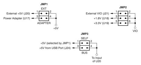
Figure 2. Power-Supply Jumper Configuration (DAIMB Motherboard)
