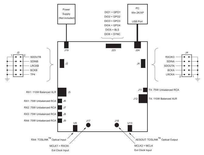
Figure 3. PDK Power, Host, and Input/Output Connections
