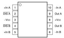
Figure 1. MSOP Package Pinout, Top View
