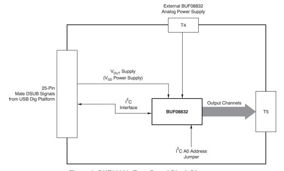
Figure 2. BUF08832\_Test\_Board Block Diagram
