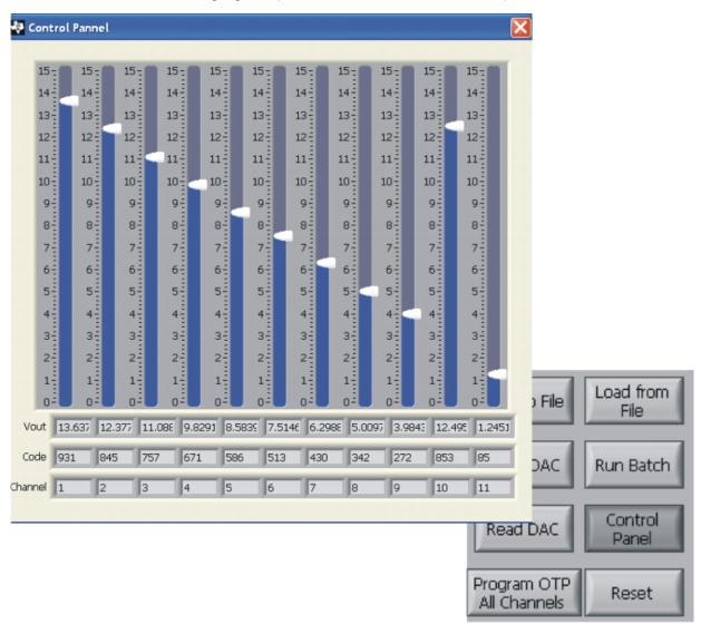
Figure 22. Control Panel Button and Window
