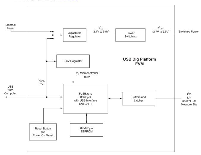
Figure 3. USB\_DIG\_Platform Theory of Operation
