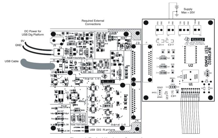
Figure 4. Typical Hardware Connections
