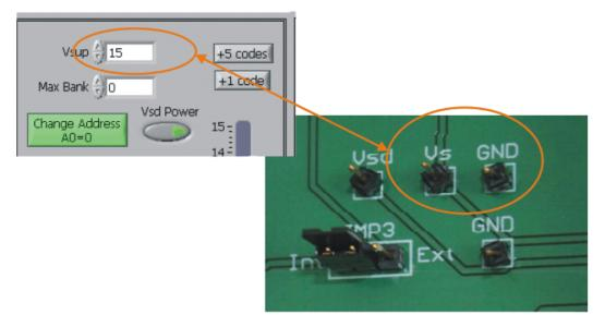
Figure 16. Measuring and Entering Power-Supply Voltage
