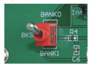
Figure 8. BKSEL Switch
