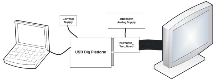
Figure 1. BUF08832EVM Hardware Setup
