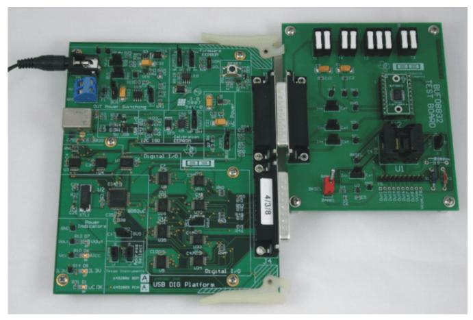
Figure 5. Connecting Power to the EVM
