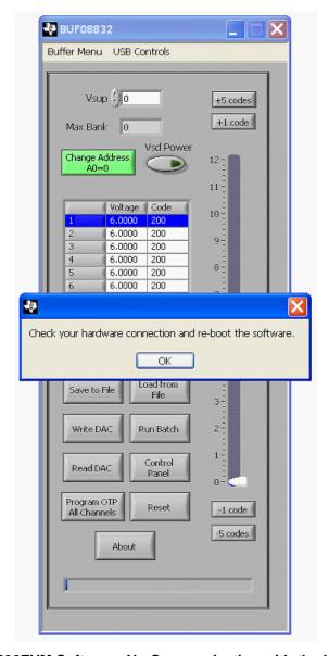
Figure 13. BUF08832EVM Software: No Communication with the USB\_DIG\_Platform
