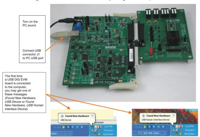
Figure 6. Connecting the USB Cable
