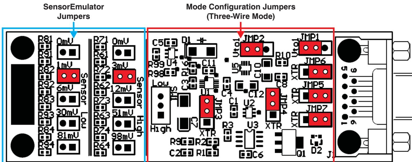
Figure 4. Jumper Setting for Voltage Output Three-Wire Mode
