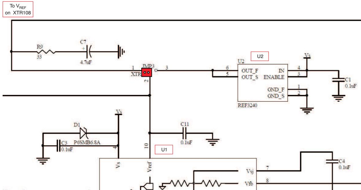
Figure 6. Reference Circuit (Configured for Current Mode)
