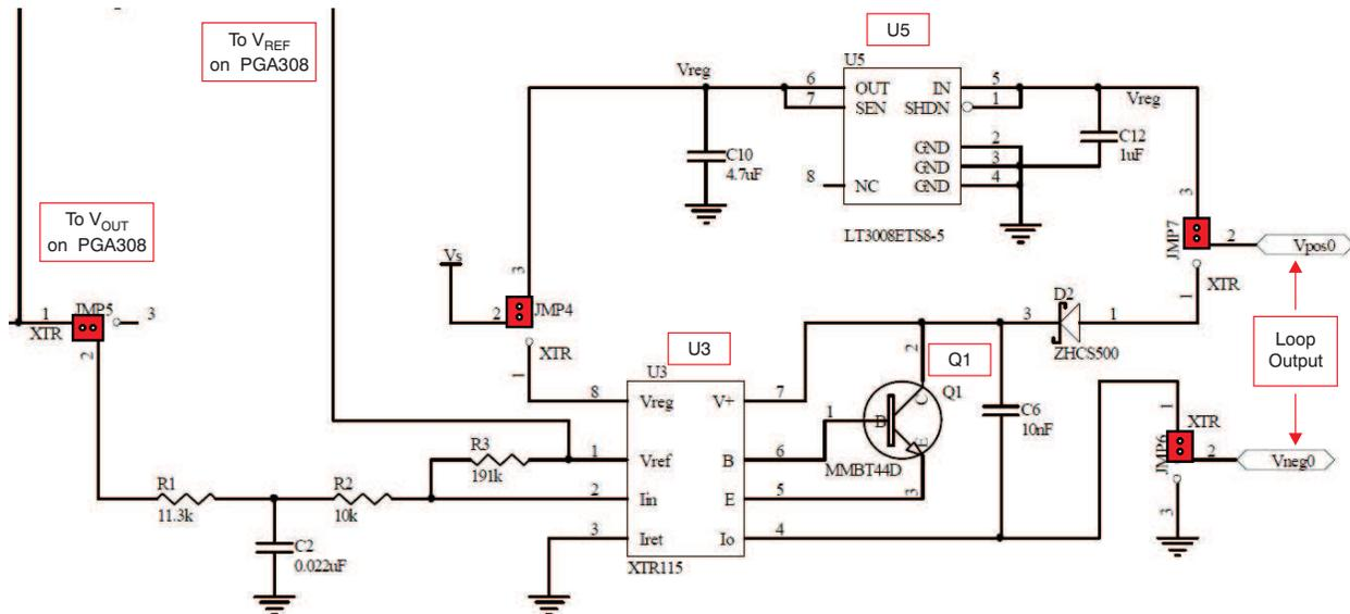
Figure 5. Current Mode Circuit (Configured for Current Mode)
