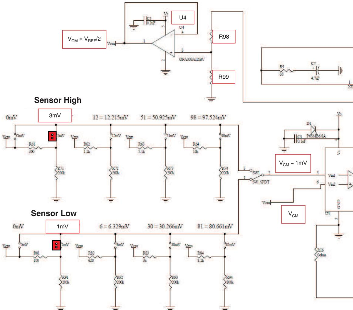
Figure 7. SensorEmulator Section (PGA308 Input)
