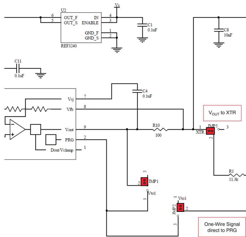
Figure 8. PGA308 Output (Configured for Current Mode)
