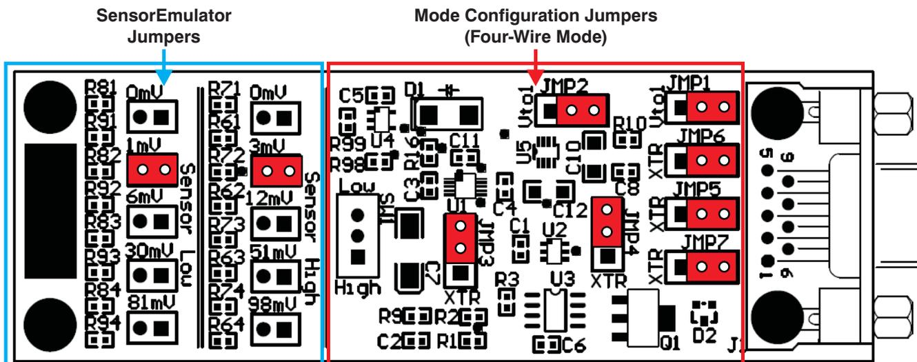
Figure 3. Jumper Setting for Voltage Output Four-Wire Mode
