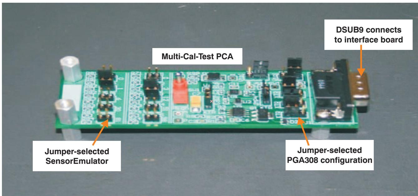
**Figure 1. Hardware Included with the Multi-Cal-Test PCA EVM Kit**
