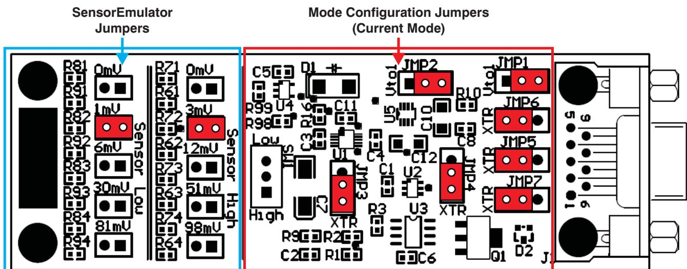
Figure 2. Jumper Settings for Current Output Mode
