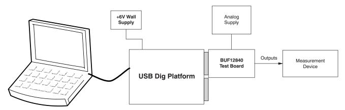
Figure 2. BUF12840EVM Hardware Setup
