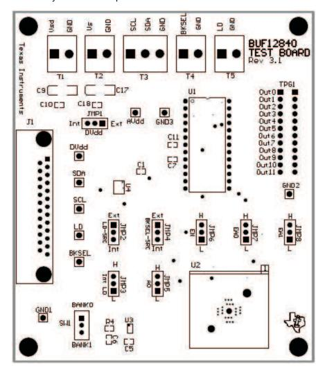
Figure 24. BUF12840EVM PCB Components Layout
