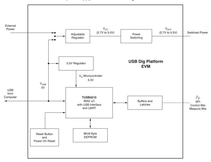
Figure 4. USB\_DIG\_Platform Theory of Operation
