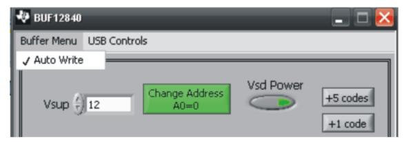
Figure 16. Auto Write Feature Enabled
