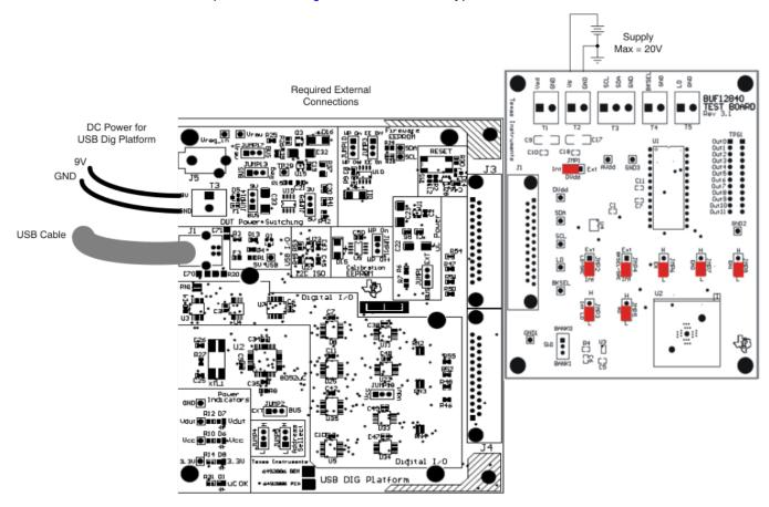
Figure 5. Typical Hardware Connections
