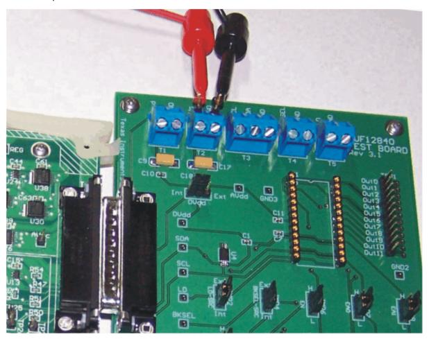
Figure 6. Connecting External Power to the EVM
