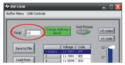
Figure 15. Measuring and Entering Power-Supply Voltage
