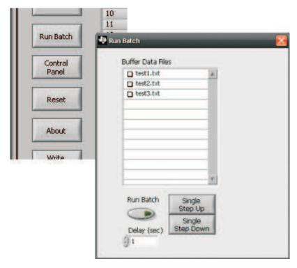
Figure 20. Run Batch Dialog Button and Window
