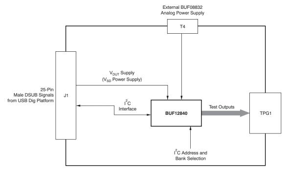
Figure 3. BUF12840 Test Board Block Diagram
