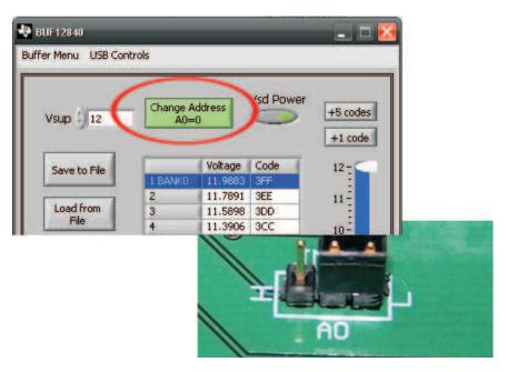
Figure 14. BUF12840 Test Board Jumper JMP5 Setting for Logic '0'
