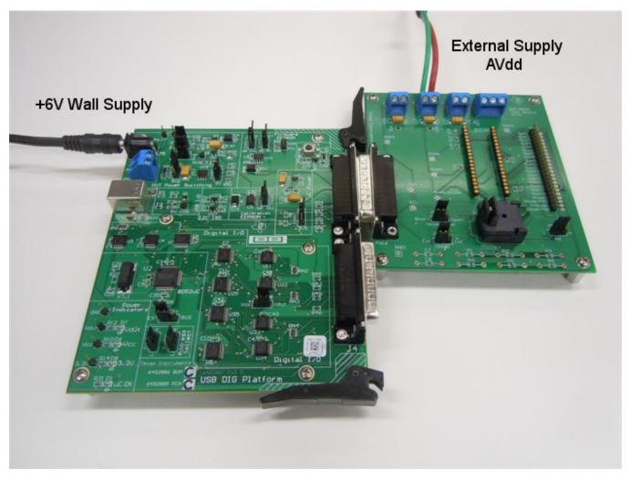
Figure 6. Connecting External Power to the EVM
