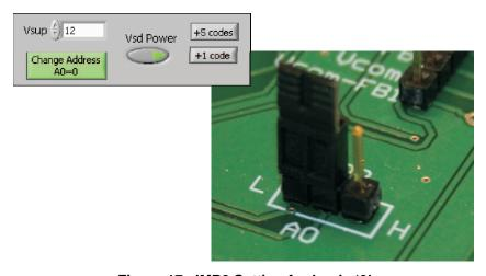
Figure 17. JMP2 Setting for Logic '0'
