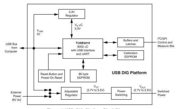
Figure 4. USB\_DIG\_Platform Block Diagram
