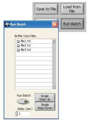
Figure 23. Run Batch Dialog Button and Window
