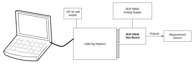
Figure 2. BUF18830EVM Hardware Setup
