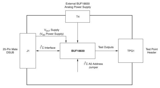
Figure 3. BUF18830EVM Board Block Diagram
