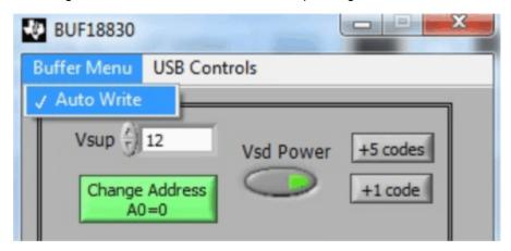
Figure 19. Auto Write Feature Enabled
