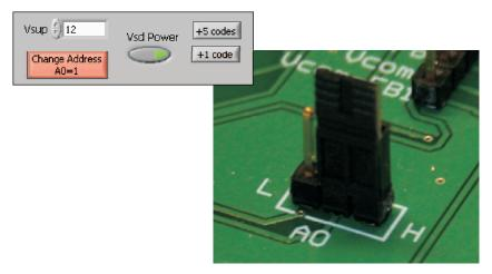
Figure 16. JMP2 Setting For Logic '1'
