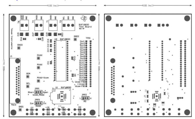
Figure 26. BUF18830EVM PCB Component Layout
