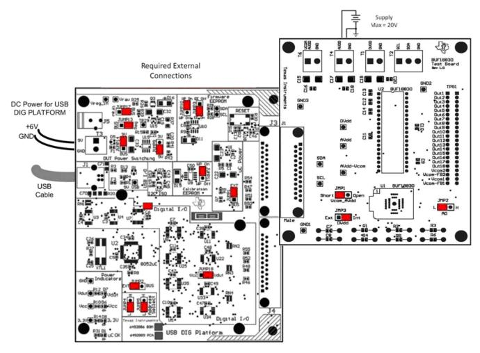
Figure 5. Typical Hardware Connections for BUF18830EVM
