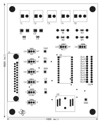
Figure 25. BUF12800EVM PCB Top Layer (Component Layout)
