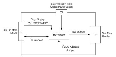
Figure 2. BUF12800EVM Board Block Diagram
