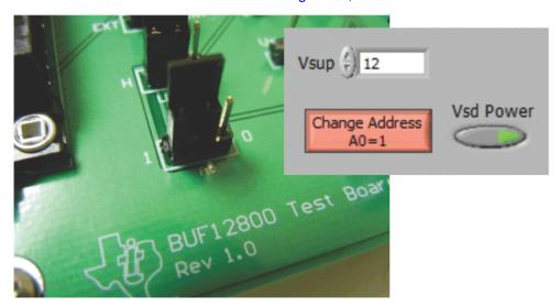
Figure 16. JMP6 Setting for Logic '1'
