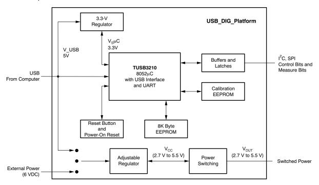
Figure 3. USB DIG Platform Block Diagram
