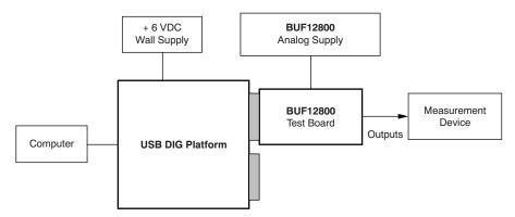
Figure 1. BUF12800EVM Hardware Setup
