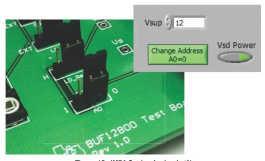
Figure 15. JMP6 Setting for Logic '0'
