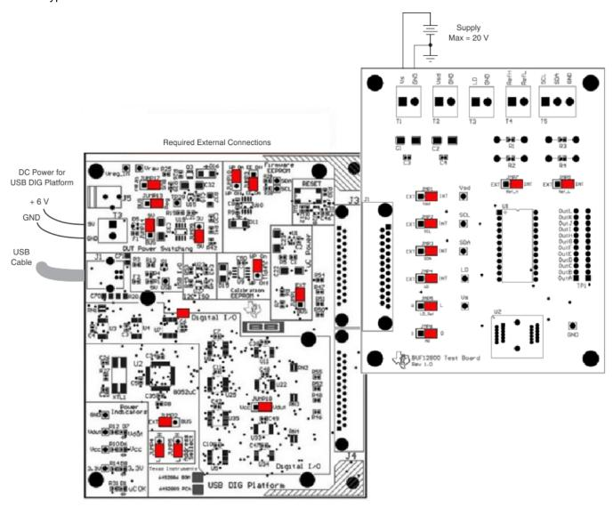
Figure 4. Typical Hardware Connections for the BUF12800EVM
