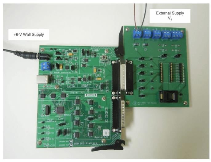
Figure 5. Connecting External Power to the BUF12800EVM
