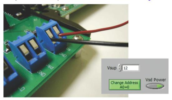
Figure 17. Measuring and Entering Power-Supply Voltage
