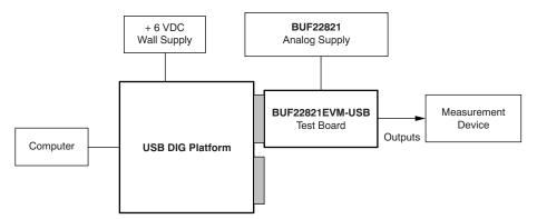
Figure 2. BUF22821EVM-USB Hardware Setup
