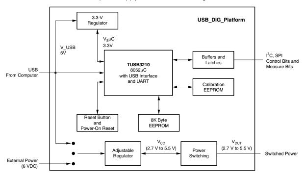
Figure 4. USB\_DIG\_Platform Block Diagram
