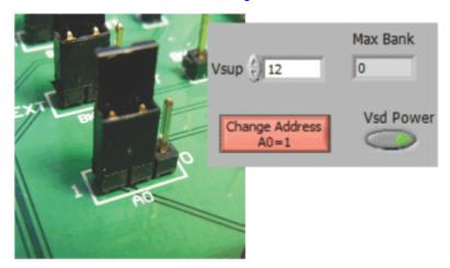
Figure 18. JMP5 Setting for Logic '1'
