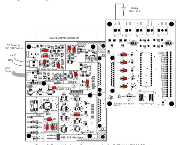
Figure 5. Typical Hardware Connections for the BUF22821EVM-USB
