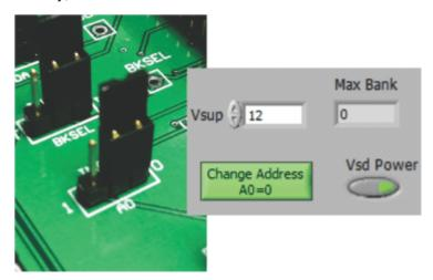
Figure 17. JMP5 Setting for Logic '0'
