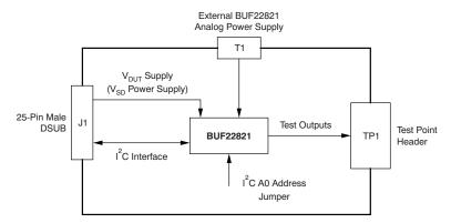
Figure 3. BUF22821EVM-USB Board Block Diagram
