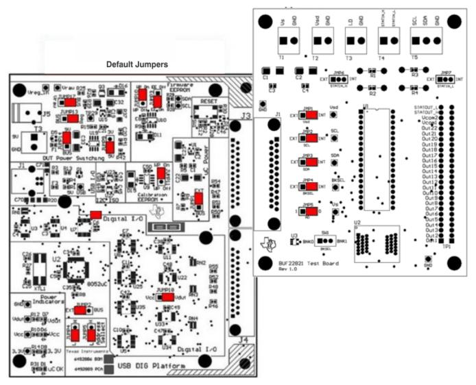
Figure 9. Default Jumper Locations for BUF22821EVM-USB
