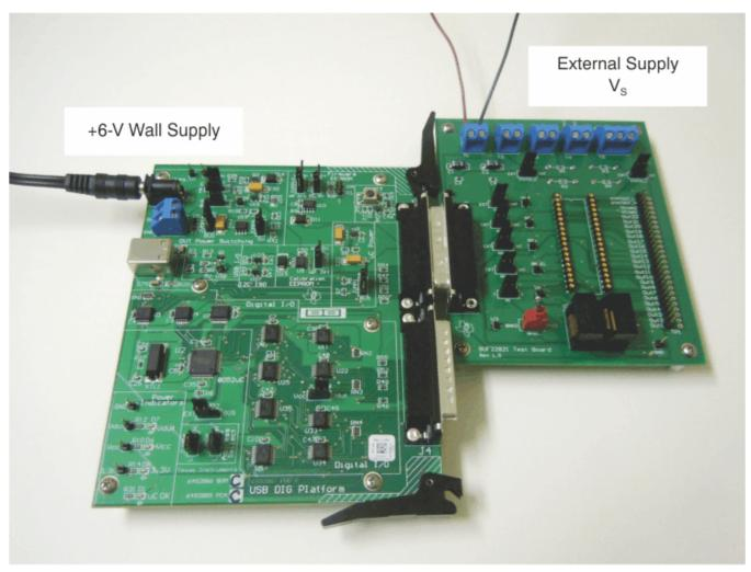
Figure 6. Connecting External Power to the BUF22821EVM-USB
