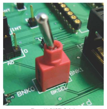
Figure 10. BKSEL Switch
