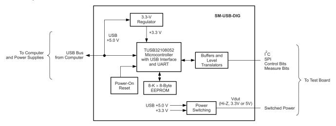
Figure 2-3. SM-USB-DIG Platform Block Diagram
