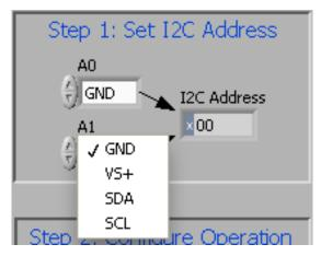
Figure 5-3. Setting the A1 Address
