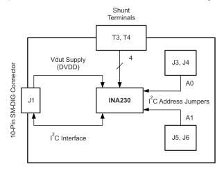
Figure 2-2. INA230EVM Test Board Block Diagram
