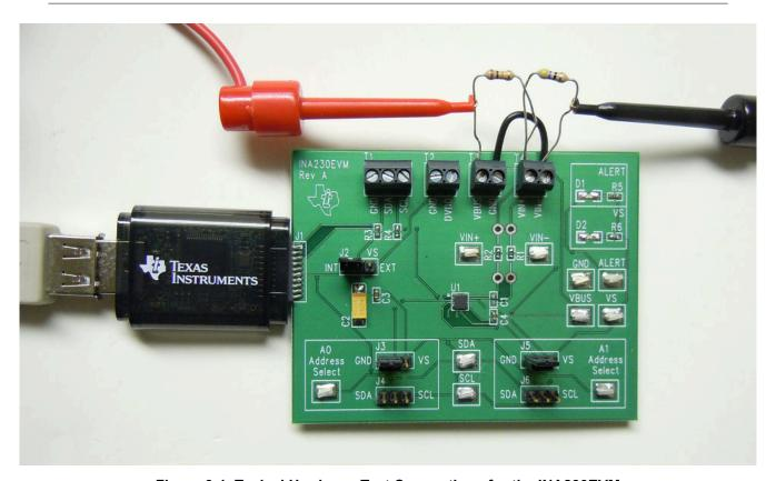
Figure 3-1. Typical Hardware Test Connections for the INA230EVM
