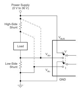
Figure 3-6. INA230 Shunt Configurations
