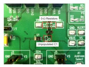
Figure 3-5. Typical Filter Setup
