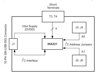
Figure 2-2. INA231EVM Test Board Block Diagram
