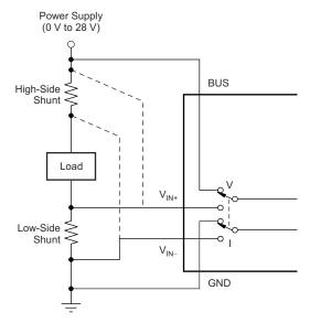
Figure 3-6. INA231 Shunt Configurations
