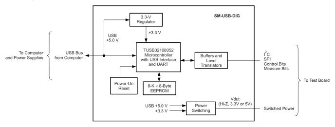
Figure 2-3. SM-USB-DIG Platform Block Diagram
