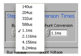
Figure 5-5. Configuring Conversion Times
