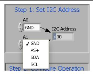
Figure 5-3. Setting the A1 Address
