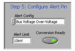
Figure 5-8. Configuring the Alert Pin
