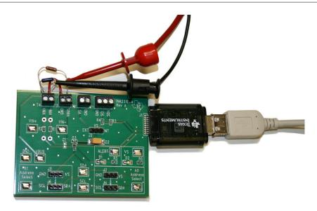
Figure 3-1. Typical Hardware Test Connections for the INA231EVM
