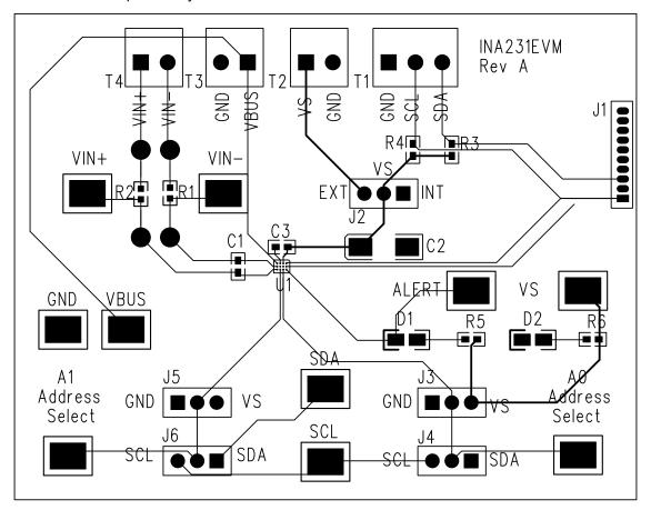
Figure 6-2. INA231EVM PCB Top Layer (Component Side)
