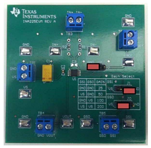
Figure 3. Jumper Configuration
