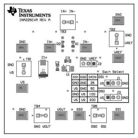
Figure 7. INA225EVM PCB Components Layout
