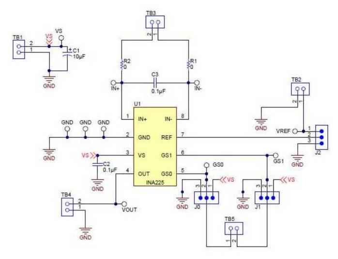
Figure 6. INA225EVM Board Schematic
