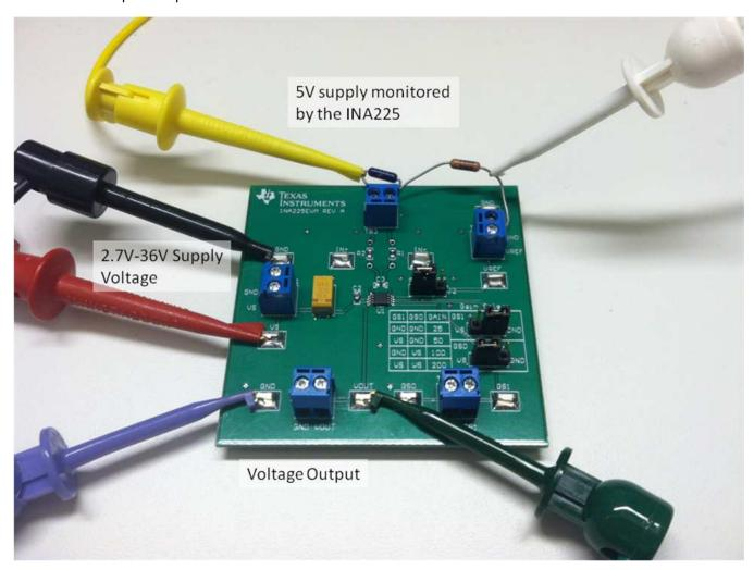
Figure 5. Basic Setup of the INA225EVM
