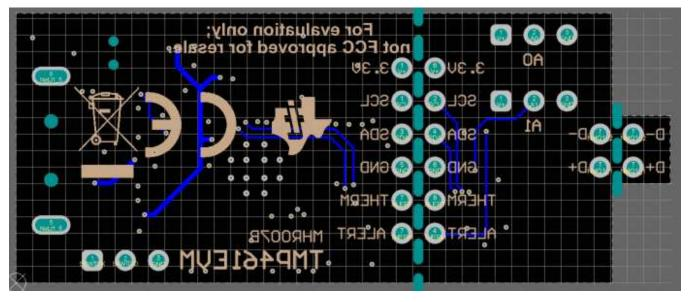
Figure 4-7. Bottom Assembly Layer
