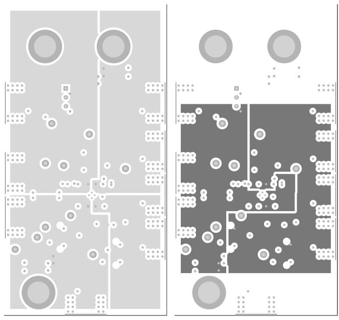
Figure 10. Layer 3: Power Plane,  $\pm V_{cc}$
