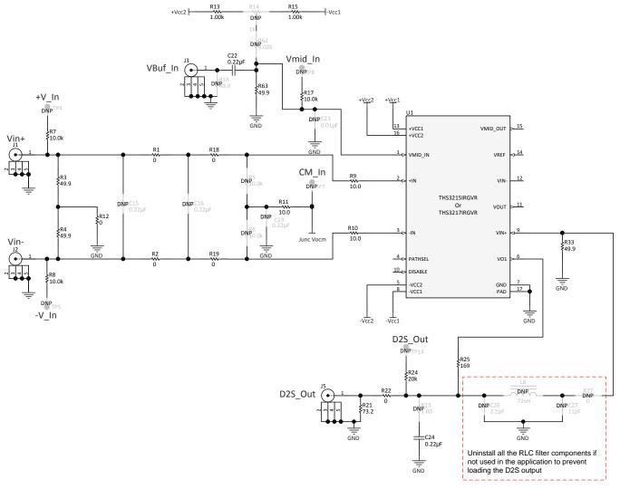
Figure 4. D2S Input Connection Options
