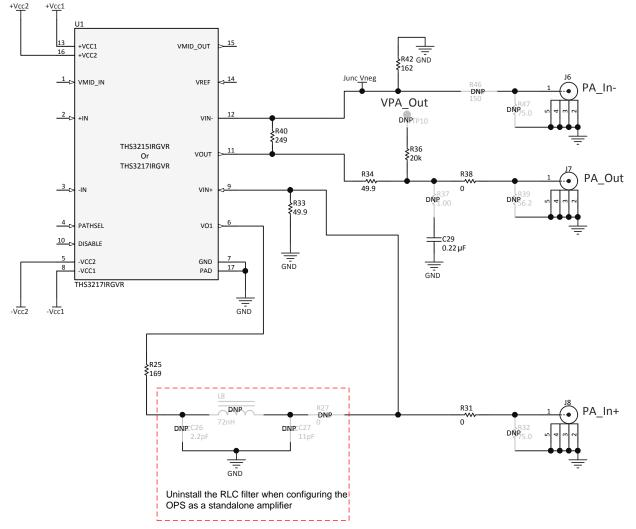
Figure 6. OPS Input and Output Connection Options
