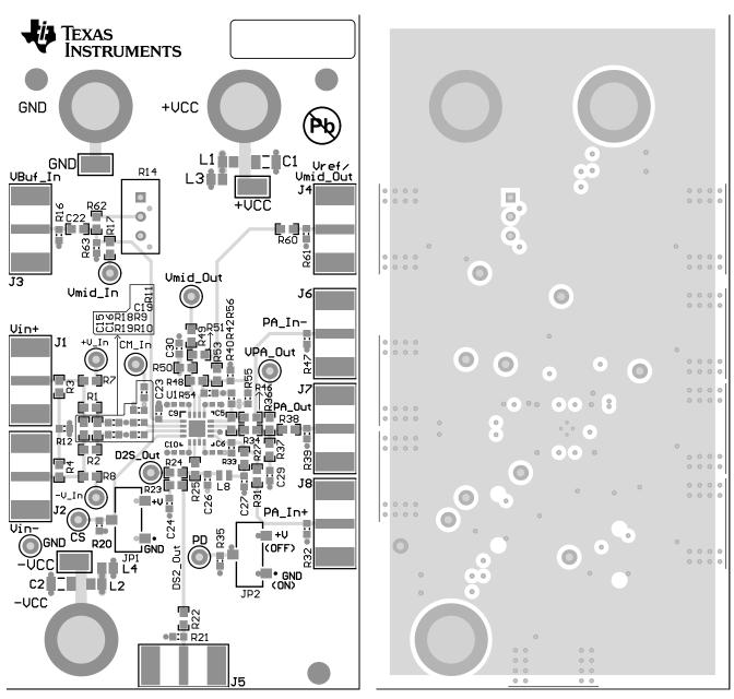
Figure 8. Layer 1: Top Signal Layer
