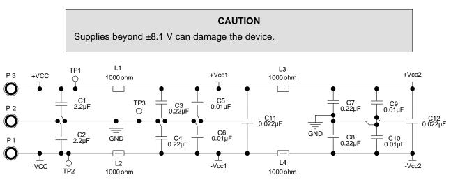
Figure 1. THS321x Power-Supply Schematic
