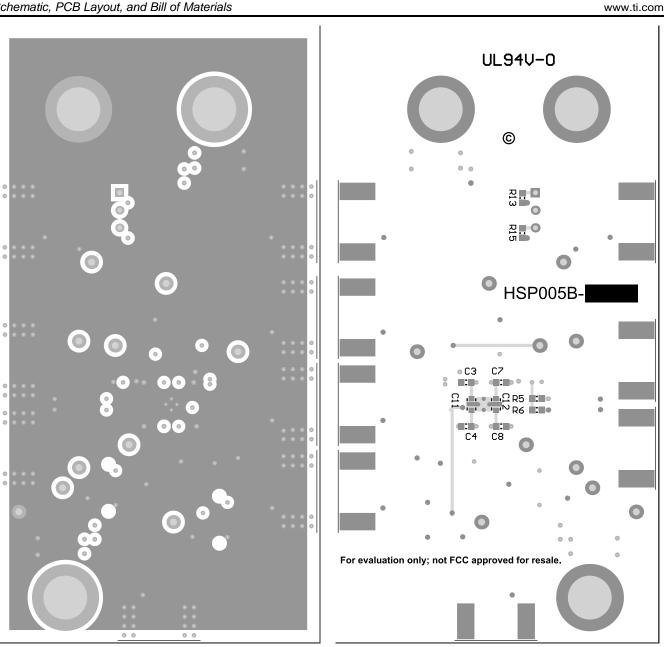
Figure 12. Layer 5: GND Plane
