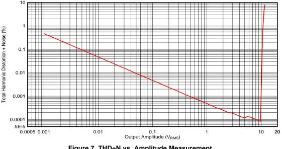
Figure 7. THD+N vs. Amplitude Measurement ±15-V Supplies, 1-kHz Output, 22-kHz MBW
