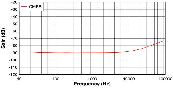
Figure 6. Common-Mode Rejection Ratio (CMRR) Measurement ±15-V Supplies, 1-V<sub>RMS</sub> Input, 90-kHz MBW
