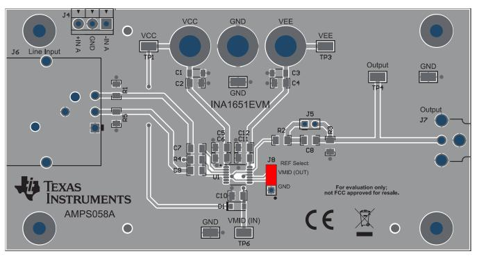
Figure 4. J8 Connection for Single-Supply Operation
