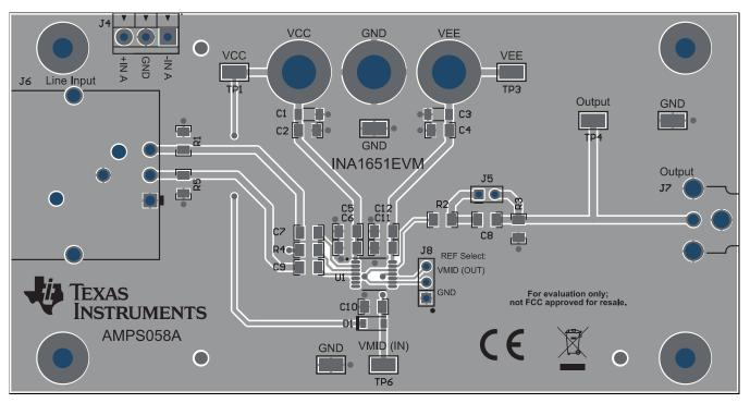
Figure 11. Top Layer PCB Layout
