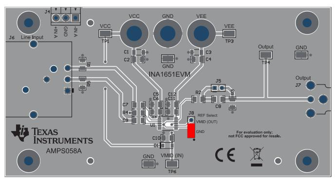
Figure 5. J8 Connection for Dual Supply Operation
