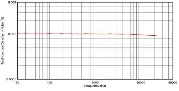
Figure 8. THD+N vs. Frequency Measurement with 1  $V_{\text{RMS}}$  Output  $\pm 15\text{-V}$  Supplies, 1-V\_{\text{RMS}} Output, 90-kHz MBW
