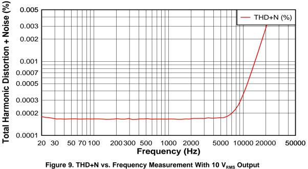
±15-V Supplies, 10-V<sub>RMS</sub> Output, 90-kHz MBW
