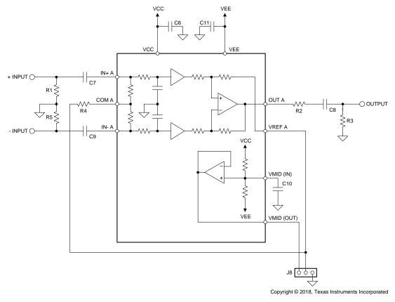
Figure 2. Simplified INA1651EVM Schematic
