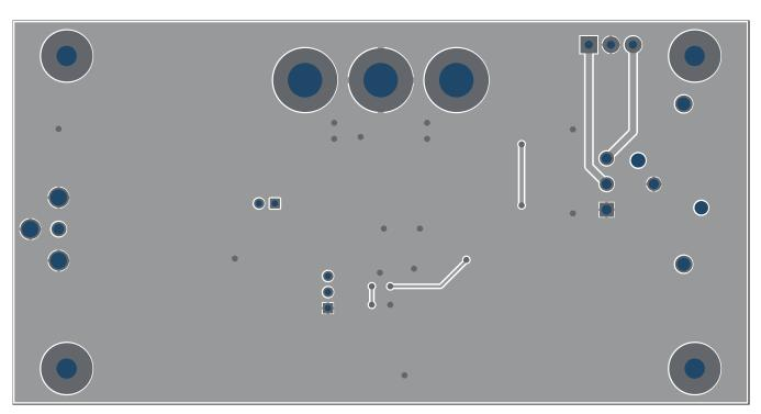
Figure 12. Bottom Layer PCB Layout
