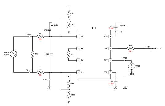
Figure 3. Single-Supply Configuration, Direct Reference Connection
