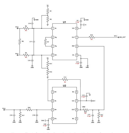
Figure 4. Single-Supply Configuration, Buffered Reference Connection
