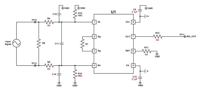
Figure 2. Dual-Supply Configuration
