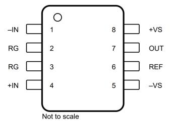
Figure 1. Universal INAEVM-ALT-SO8 Pinout
