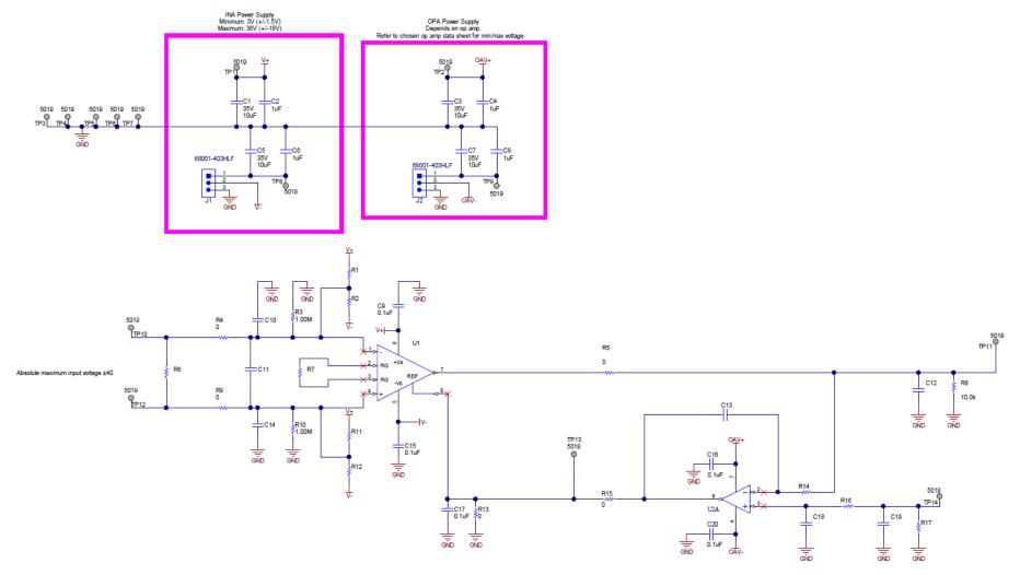
Figure 5. Universal INAEVM-ALT-SO8 Schematic (1)
