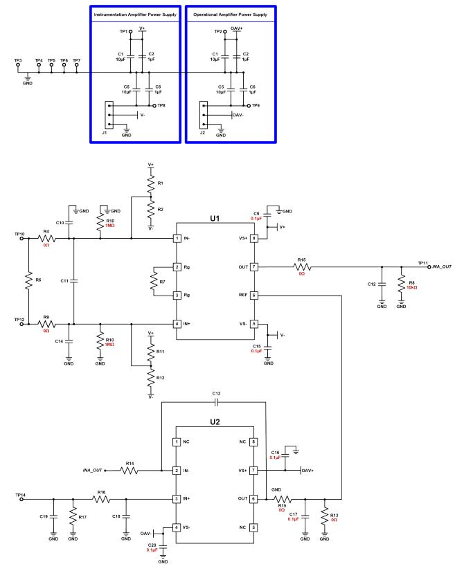
Figure 6. Universal INAEVM-ALT-SO8 Schematic (2)
