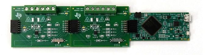
Figure 4-2. Multiple EVMs Connected to SCB Controller
