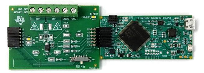
Figure 4-1. EVM (Left) Connected to SCB Controller (Right)
