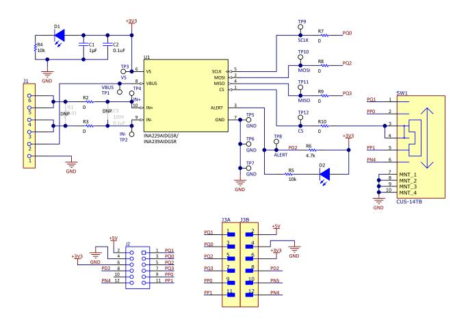
Figure 6-3. SENS064 Schematic
