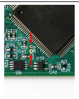
Figure 4-3. Test Points Used to Enter DFU Mode Manually
