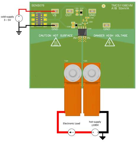
Figure 4-1. Low-Side Forward Current Setup
