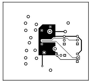
Figure 5-14. INA2191EVM Bottom Layer for Single Panel
