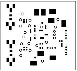
Figure 5-15. INA2191EVM Top Solder for Single Panel
