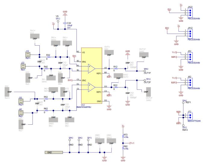
Figure 5-2. INA2191EVM Schematic: Gain A2 Panel
