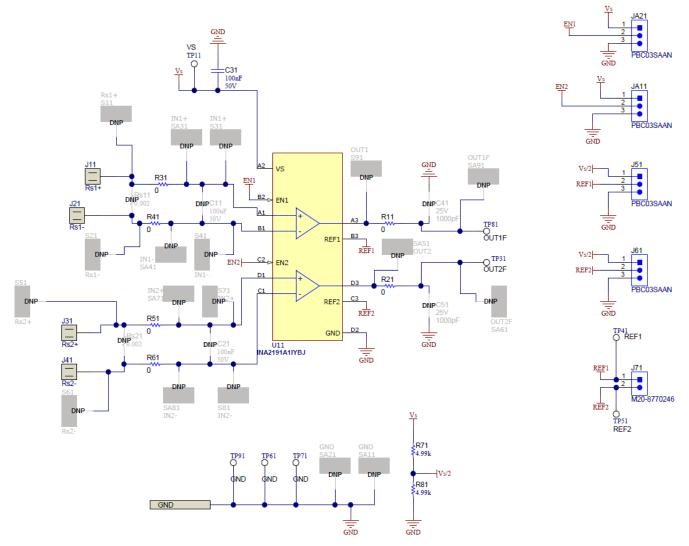
Figure 5-1. INA2191EVM Schematic: Gain A1 Panel
