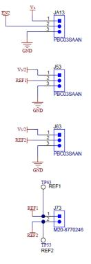
Figure 5-3. INA2191EVM Schematic: Gain A3 Panel
