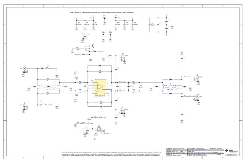
Figure 8-1. LMH5485-SP Recommended Default Schematic
