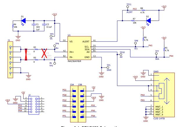
Figure 6-1. SENS079 Schematic
