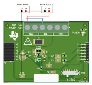
Figure 4-14. IN+ and IN- Wiring Without a Shunt Resistor
