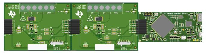
Figure 4-2. Multiple EVMs Connected to SCB Controller
