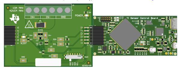
Figure 4-1. EVM Connected to SCB Controller
