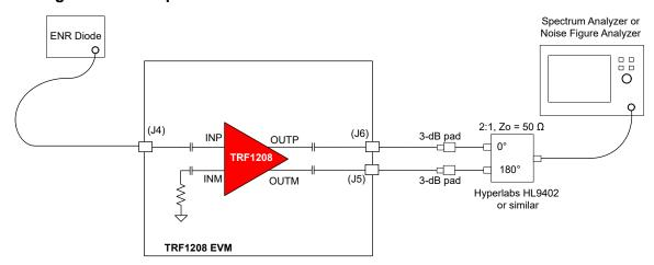
Figure 3-3. Noise Figure Test Setup
