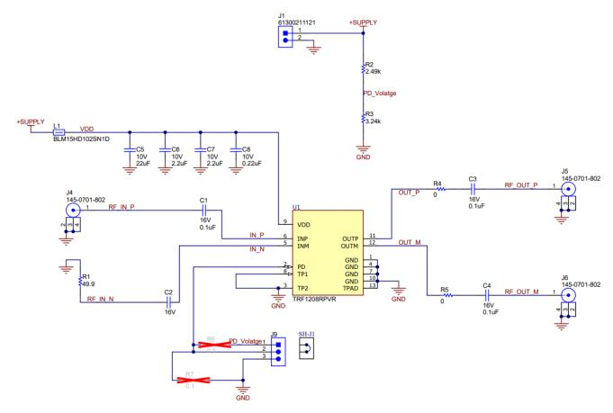
Figure 2-1. TRF1208 EVM Schematic
