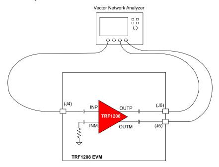
Figure 3-1. S-Parameter Test Setup
