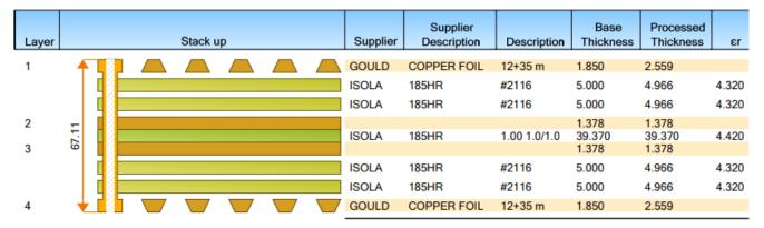
Figure 2-6. TRF1208 EVM Stack-Up (Units in Mils)
