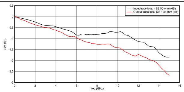
Figure 3-2. PCB Trace Loss vs Frequency
