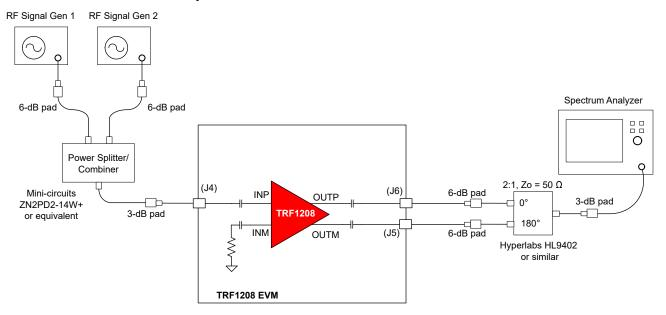
Figure 3-4. OIP3 Test Setup
