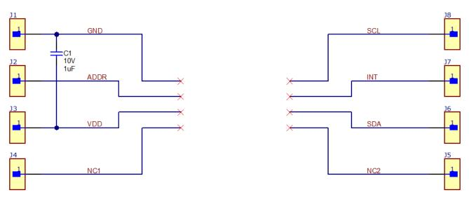
Figure 4-7. OPT4001 Coupon Rigid Board Schematic
