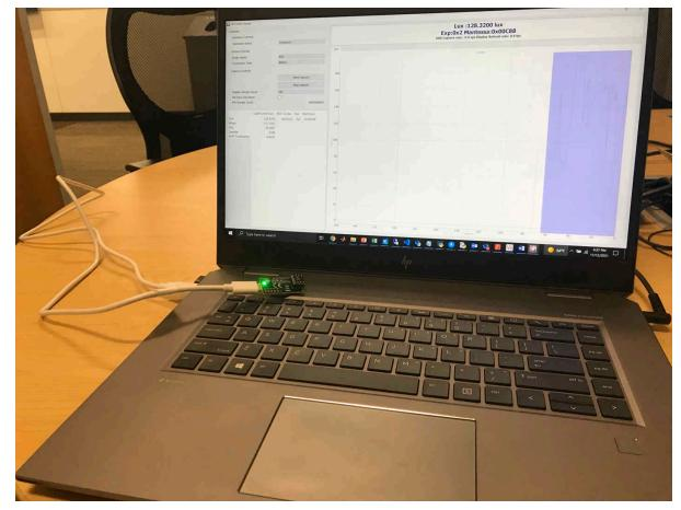
Figure 2-1. EVM Hardware Setup
