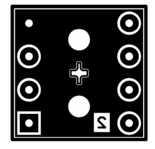
Figure 4-4. PCB Bottom Layer
