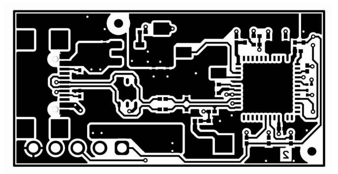
Figure 4-14. PCB Bottom Layer
