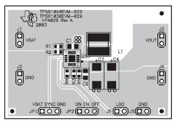
Figure 3-2. Top Layer Routing
