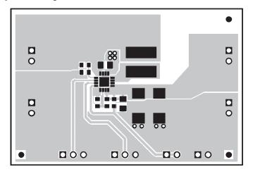
Figure 3–3. Bottom Layer Routing
