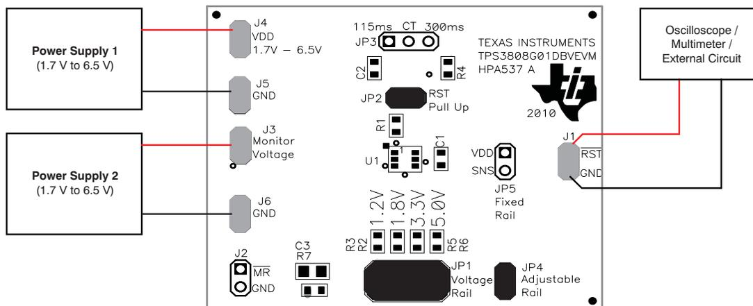
Figure 2. Using the TPS3808G01EVM as a Dual-Rail Monitor
