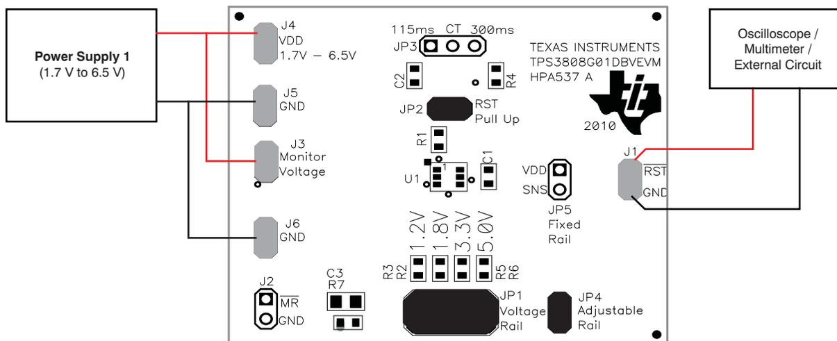
**Figure 1. Using the TPS3808G01EVM as a Single-Rail Monitor**
