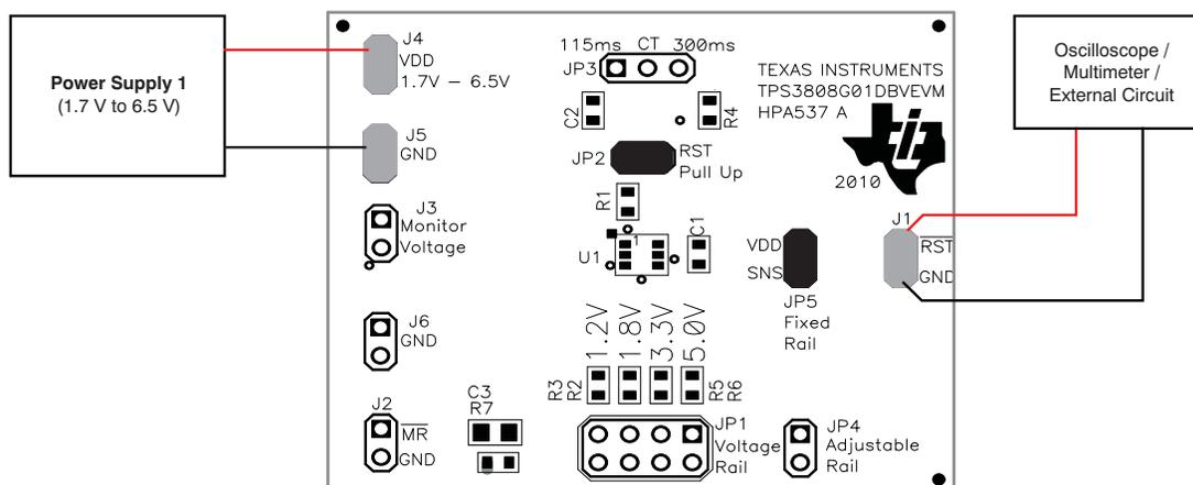
Figure 3. Using the TPS3808G01EVM with Fixed-Voltage TPS3808Gxx
