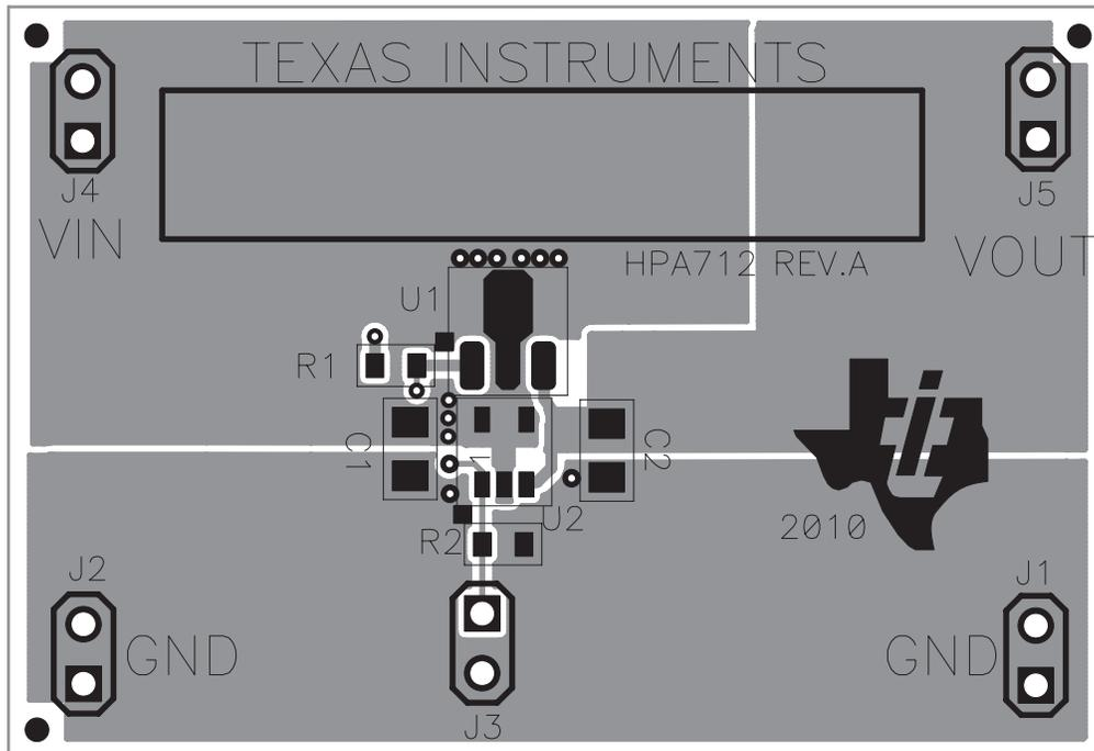
**Figure 3. Assembly Layer**
