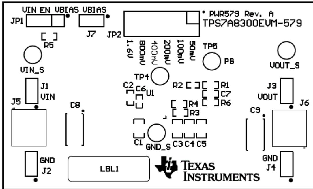
Figure 1. Assembly Layer
