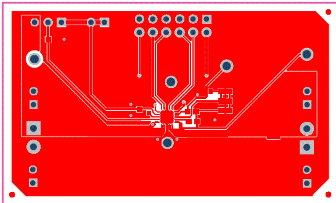
Figure 2. Top Layer Routing
