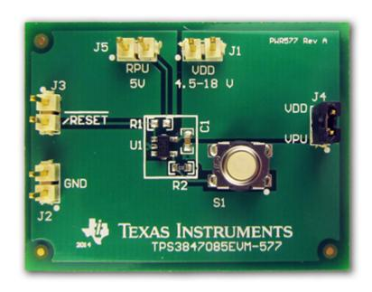
This user's guide describes the operational use of the TPS3847085EVM-577 evaluation module (EVM) as a reference design for engineering demonstration and evaluation of the TPS3847085, an ultralow-power, wide supply voltage, supervisory circuit. Included in this user's guide are setup instructions, a schematic diagram, printed circuit board (PCB) layout drawings, and a bill of materials for the EVM.
