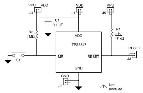
Figure 4. TPS3847085EVM-577 Schematic
