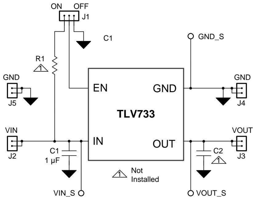
Figure 6. TLV73312PDQN-643 Schematic
