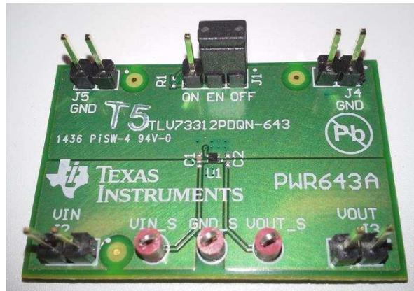
This user's guide describes the operational use of the TLV73312PDQN-643 evaluation module (EVM) as a reference design for engineering demonstration and evaluation of the [TLV73312PDQN](#), an ultra-small, low-quiescent current, low-dropout regulator (LDO). Included in this user's guide are setup instructions, a schematic diagram, printed circuit board (PCB) layout drawings, and a bill of materials for the EVM.
