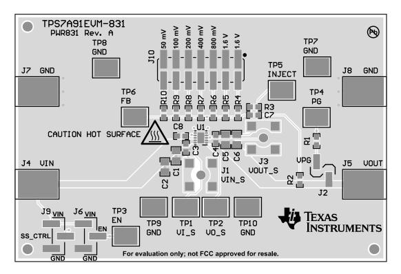
Figure 1. Assembly Layer
