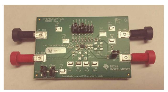
This user's guide describes the operational use of the TPS7A91EVM-831 evaluation module (EVM) as a reference design for engineering demonstration and evaluation of the TPS7A9101DSK, low-dropout linear regulator (LDO). Included in this user's guide are setup and operating instructions, thermal and layout guidelines, a printed-circuit-board (PCB) layout, a schematic diagram, and a bill of materials (BOM).
