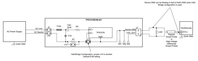
Figure 2-2. Proper Test Equipment Connections for the Half-Bridge (HB) EVM Configuration
