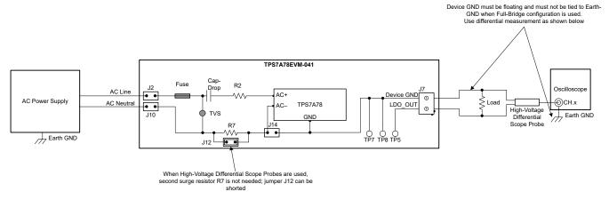
Figure 2-1. Proper Test Equipment Connections for the FB EVM Configuration
