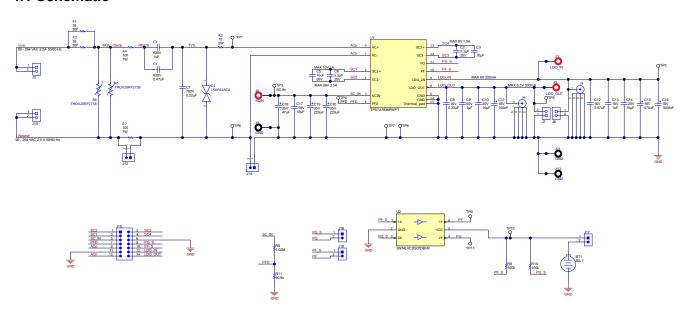
Figure 4-1. TPS7A78EVM-041 Schematic
