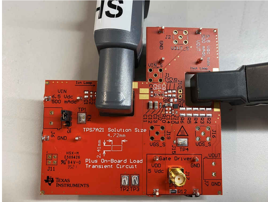
Figure 3-2. TPS7A21EVM-059 With Current Probes Attached
