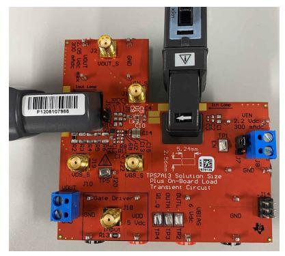
Figure 3-2. TPS7A13EVM-057 With Current Probes Attached
