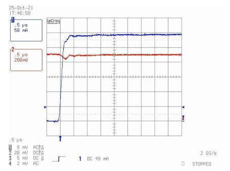
Figure 3-3. TPS7A13EVM-057 Load Transient Results: 1-mA to 300-mA Load Step
