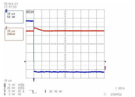
Figure 3-4. TPS7A13EVM-057 Load Transient Results: 300-mA to 1-mA Load Step
