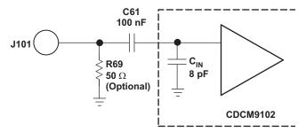
Figure 3. Single-Ended Connection Configuration
