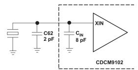
NOTE: This configuration assumes that the crystal is placed very close to the XIN pin on the device.
