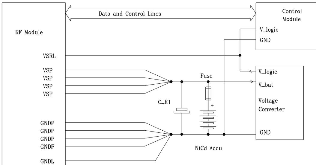
**Figure 5-2. Supply Line Wiring for Short Supply Lines**
