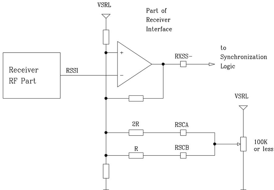
**Figure 5-5. Synchronization Output Control - Analog Adjustment**
