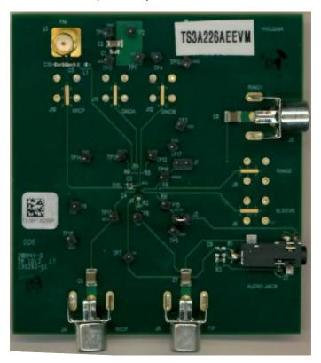
Figure 1. TS3A226AE Evaluation board
