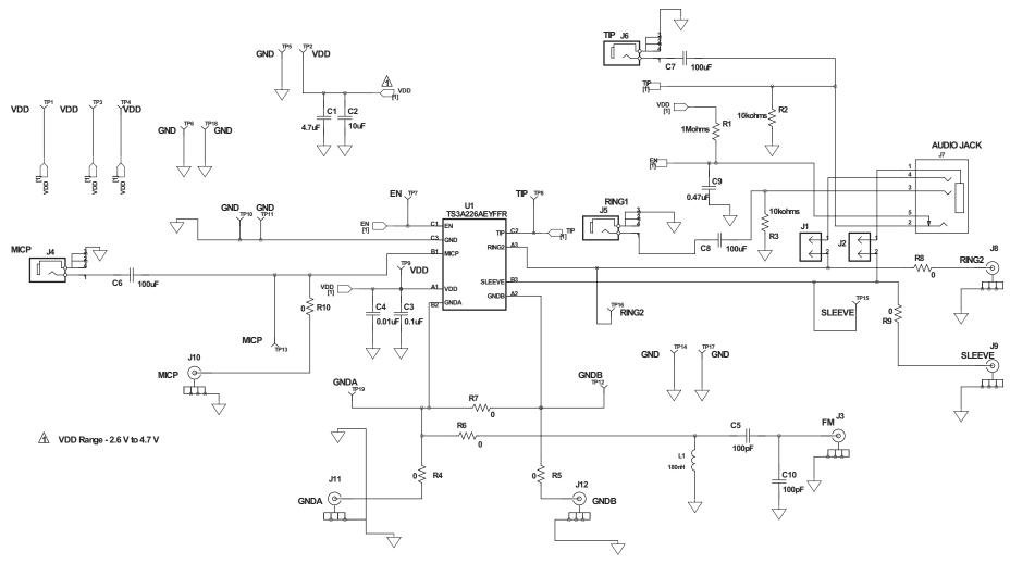
Figure 2. TS3A226AE EVM Schematic
