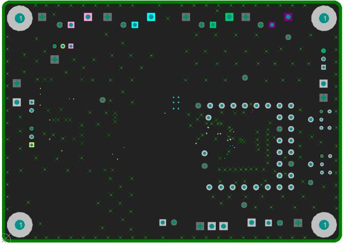
Figure 18. TS3DDR32611 EVM Internal Layer 1 (GND Layer)
