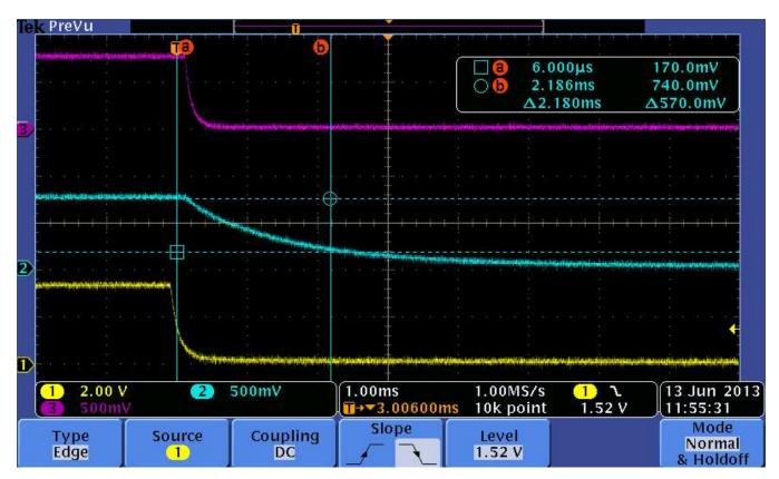
Figure 13. ODT\_EN Enable Turn off
