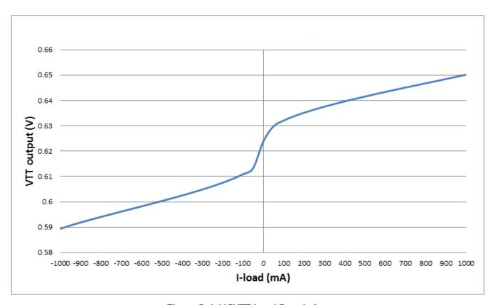
Figure 5. 0.625VTT Load Regulation
