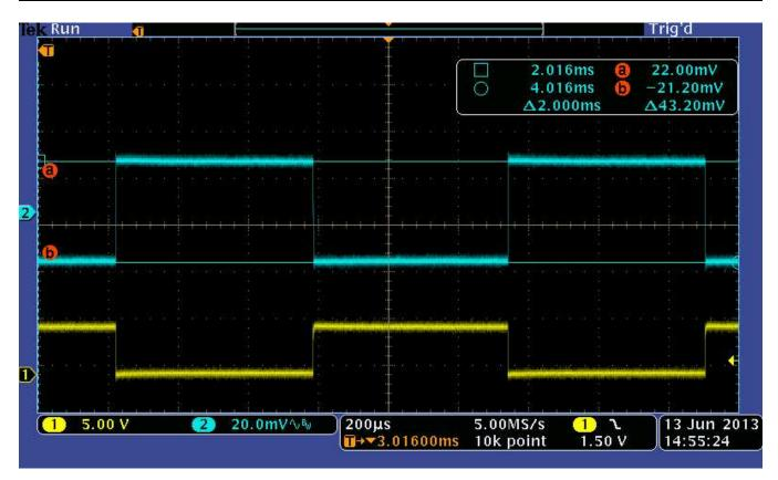
Figure 10. 0.675VTT 615mA Sink/Source
