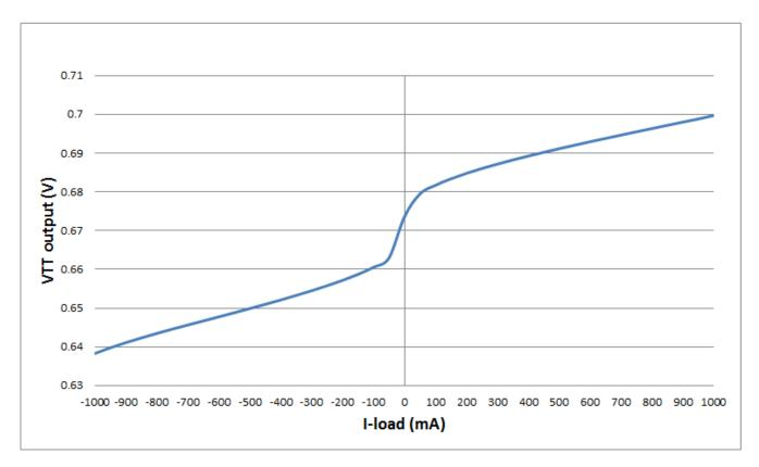
Figure 4. 0.675VTT Load Regulation
