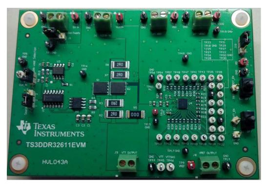
Figure 1. TS3DDR32611 Evaluation board
