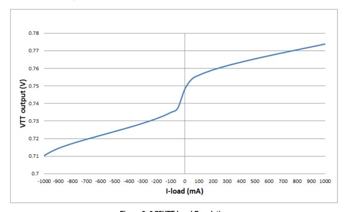
Figure 3. 0.75VTT Load Regulation
