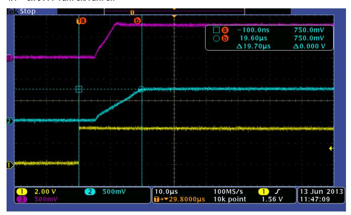
Figure 12. ODT\_EN Enable Turn on
