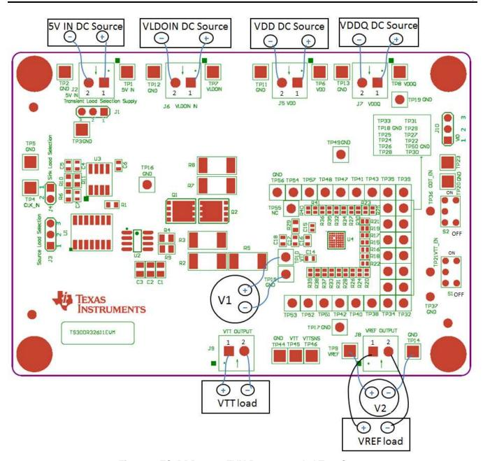
Figure 2. TS3DDR32611 EVM Recommended Test Setup
