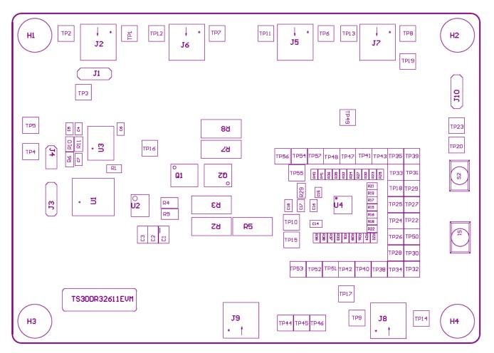
Figure 16. TS3DDR32611 EVM Top Layer Assembly Drawing
