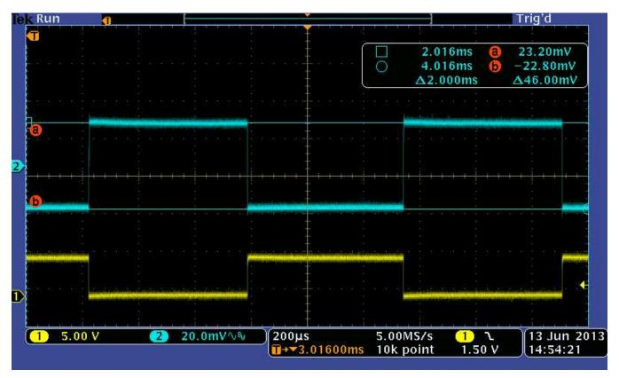
Figure 9. 0.75VTT 685mA Sink/Source
