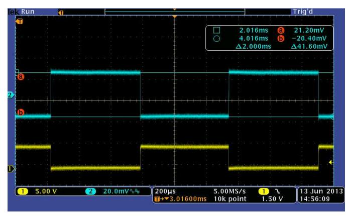
Figure 11. 0.625VTT 570mA Sink/Source
