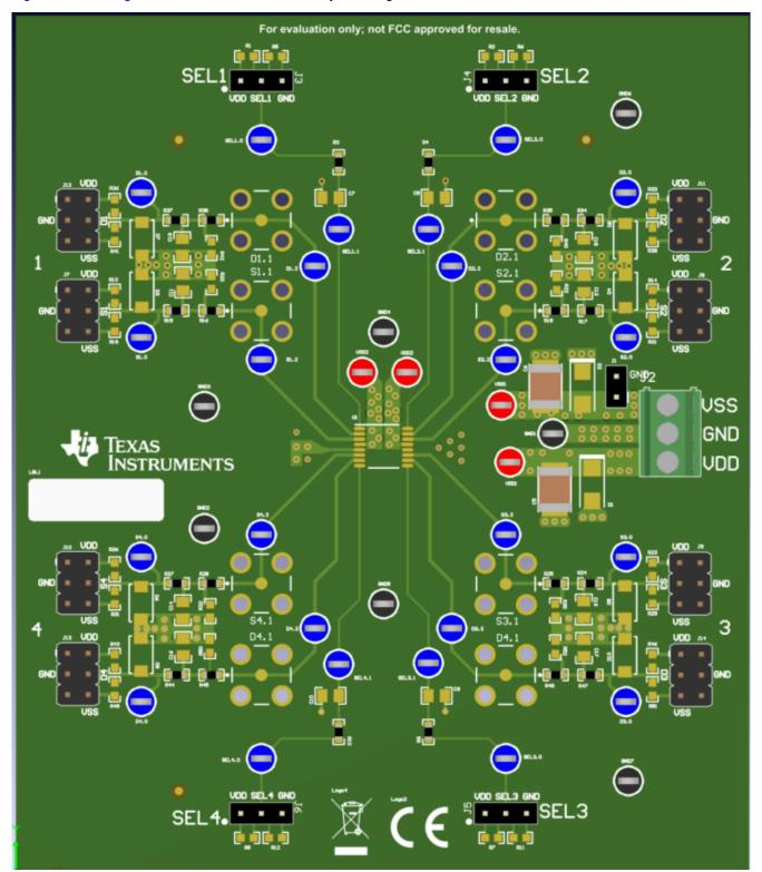
Figure 7-1. Top View Illustration of the TMUX721xEVM Layout
