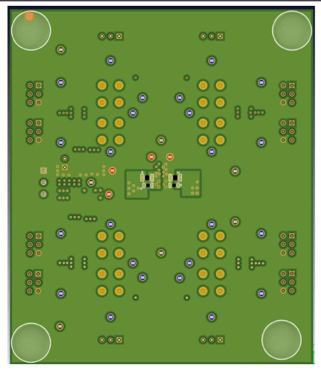
Figure 7-2. Bottom View Illustration of the TMUX721xEVM Layout
