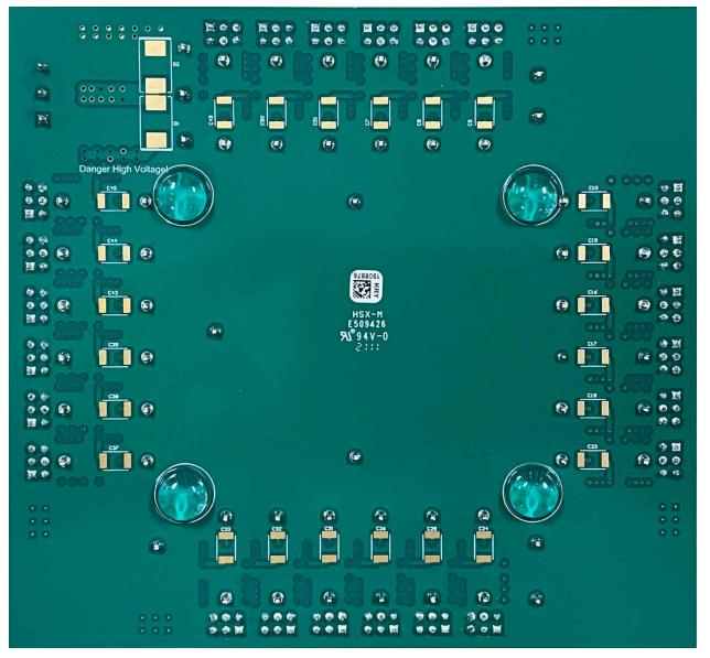
Figure 1-2. TMUX-24PW-EVM Bottom View
