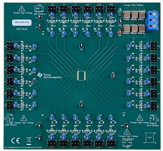
Figure 1-1. TMUX-24PW-EVM Top View
