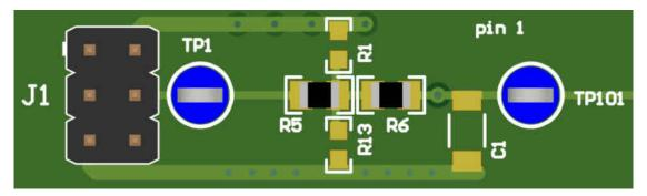
Figure 6-3. Signal Line Circuitry
