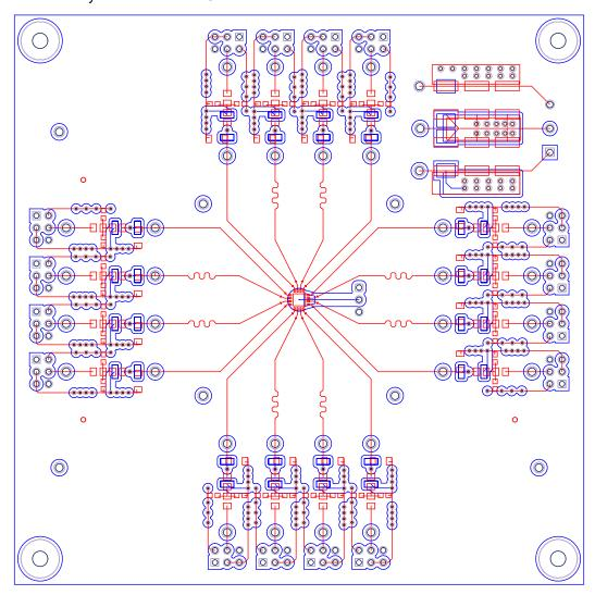
Figure 7-1. Illustration of TMUXRUM-RRPEVM Layout
