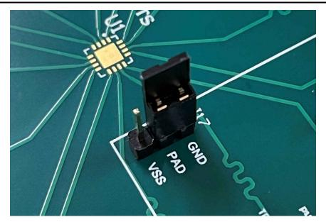
Figure 6-5. Thermal Pad Selector with Shunt
