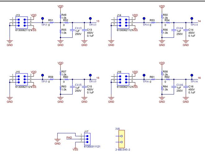
In assembly, connect J18 between pins 1 and 2 of J17.
