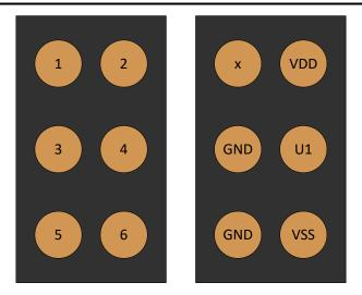
Figure 5-2. Pinout of Headers
