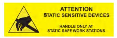
This EVM contains components that can potentially be damaged by electrostatic discharge. Always transport and store the EVM in its supplied ESD bag when not in use. Handle using an antistatic wristband. Operate on an antistatic work surface. For more information on proper handling, see Electrostatic Discharge (ESD).
