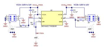
Figure 3-2. Schematic - One Channel DEA
