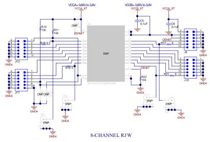
Figure 3-4. Schematic - Eight Channel RJW
