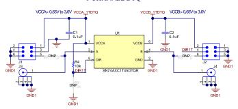
Figure 3-1. Schematic - One Channel DTQ
