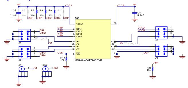
Figure 3. SN74AXC4T774EVM RSV Schematic
