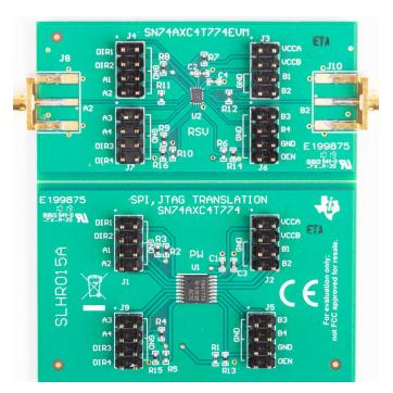
Figure 1. SPI/JTAG Translation using SN74AXC4T774EVM
