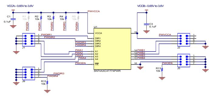
Figure 4. SN74AXC4T774EVM PW Schematic
