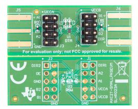
Figure 1. AXC2T-SMALLPKGEVM with DTM and RSW packages
