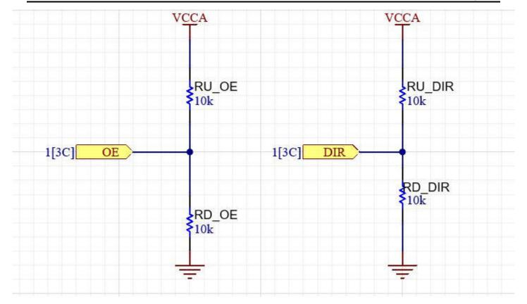
Figure 3-5. TXV0108-EVM Control Inputs
