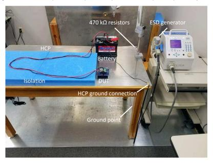
Figure 6. Powered-up Setup
