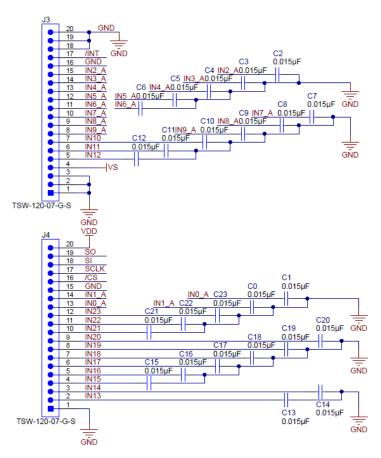
Figure 2. TIC12400-Q1 and TIC10024-Q1 Test Board Schematic Part 1
