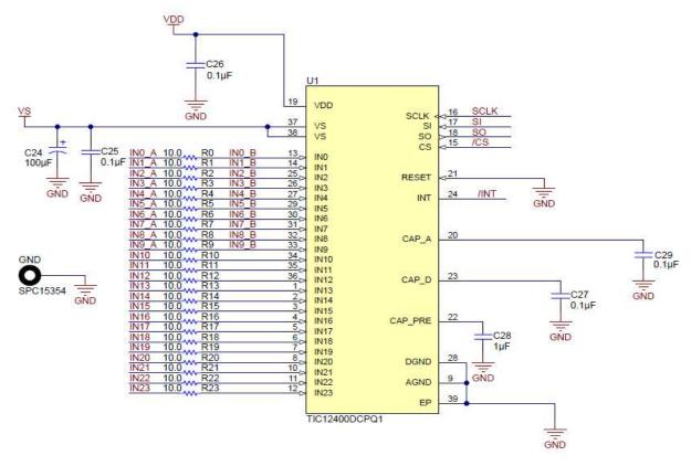
Figure 1. TIC12400-Q1 and TIC10024-Q1 Test Board Schematic Part 1
