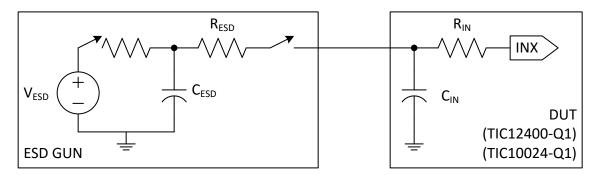
Figure 4. ESD Gun and DUT Equivalent Circuit
