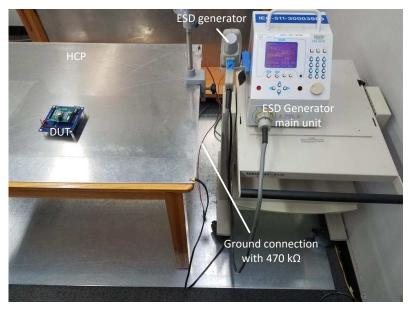
Figure 7. Unpowered Setup
