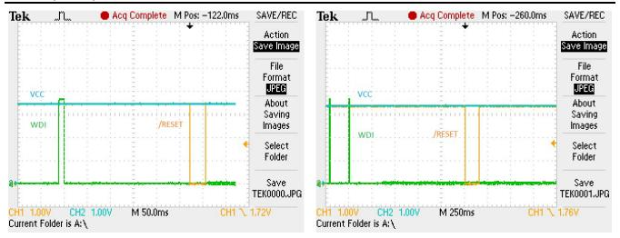
Figure 17. TPS3820-33-Q1 Watchdog Timeout t<sub>tout</sub>, From WDI Falling to RESET Falling
