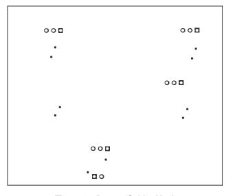
Figure 10. Bottom Solder Mask
