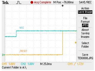
Figure 13. TPS3828-33-Q1 RESET De-Asserted Due to Rising VCC, With Delay t<sub>d</sub>
