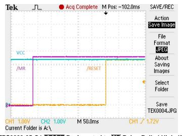
Figure 16. TPS3823-25-Q1 RESET De-Asserted to MR Being Pulled High, With Delay t<sub>d</sub>
