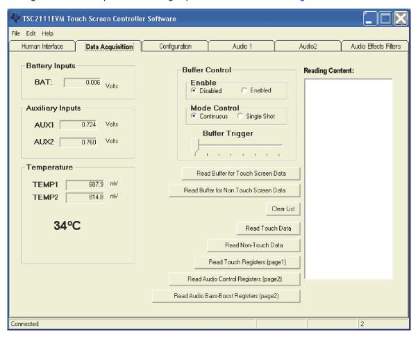
Figure 5. Data Acquisition Screen
