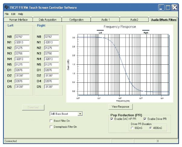
Figure 12. Bass Boost Filter Screen Default Configuration
