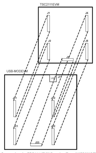
Figure 1. Connecting the TSC2111EVM Board to Top of USBMODEVM Board
