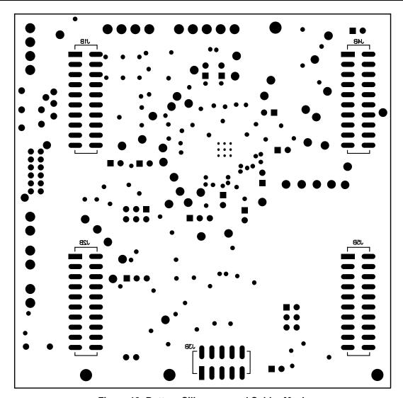
Figure 19. Bottom Silkscreen and Solder Mask
