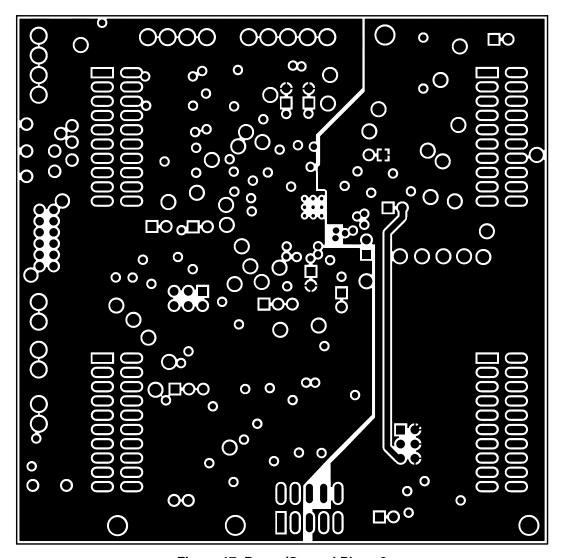
Figure 17. Power/Ground Plane 2
