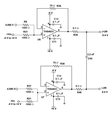
Figure 1. Input Buffer, Bipolar Fully Differential Input
