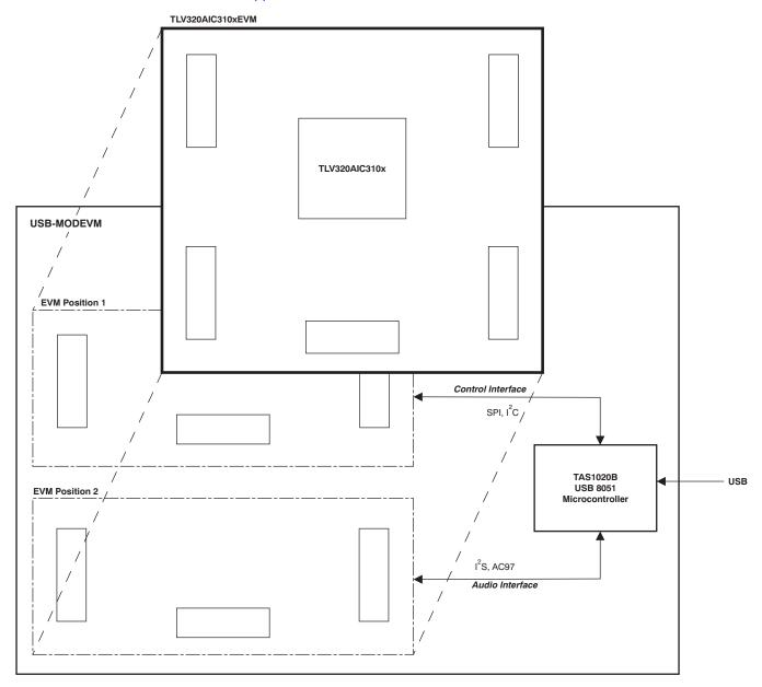
Figure 1. TLV320AlC3105EVM-PDK Block Diagram
