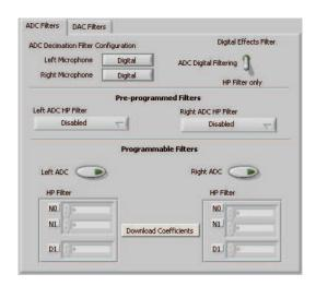
Figure 13. ADC High-Pass Filters
