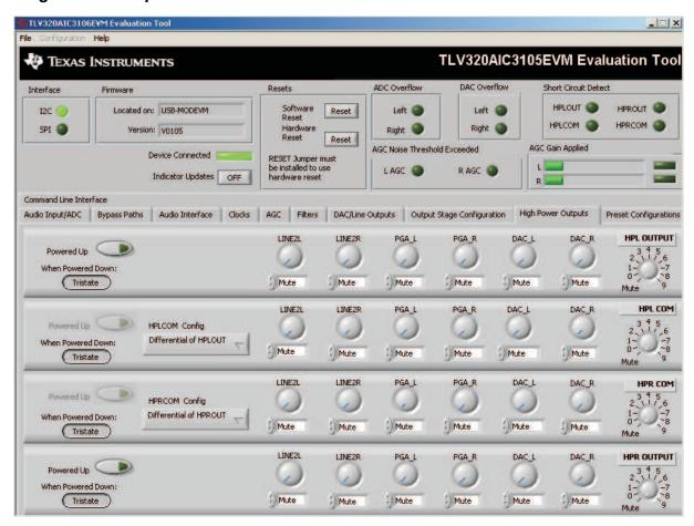
Figure 26. High Power Outputs Tab
