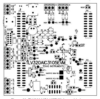
Figure 29. TLV320AIC3105EVM Assembly Layer
