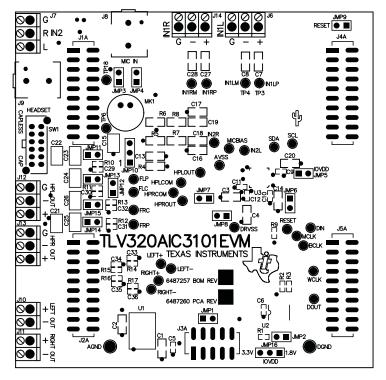
Figure 31. TLV320AIC3101EVM Assembly Layer
