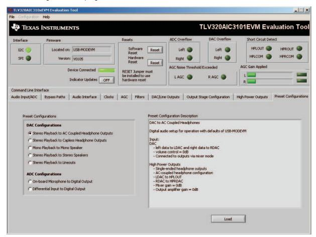
Figure 4. Default Configuration Tab
