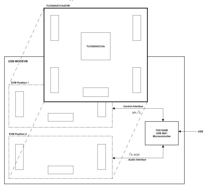
Figure 1. TLV320AIC3101EVM-PDK Block Diagram
